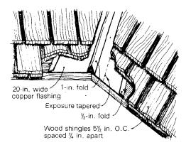
derneath-the water can't jump the crimps so it runs back down the valley toward the gutter.
