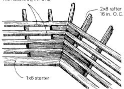
weather, my 1x3s are also spaced 51/2 in., except in the valleys, where I butt strips together to create a solid base for the flashing that follows.
