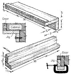
kickspace and push it tight against the underside of the cabinet edge. To hold the jig in place, screw its back edge to the plinth (the screw holes will be covered by a kick strip) or wedge the jig tight with scraps built up from the floor. With the bottoms of your doors resting on this level jig, you need worry only about the doors' left-right positioning; all their heights will be the same.
